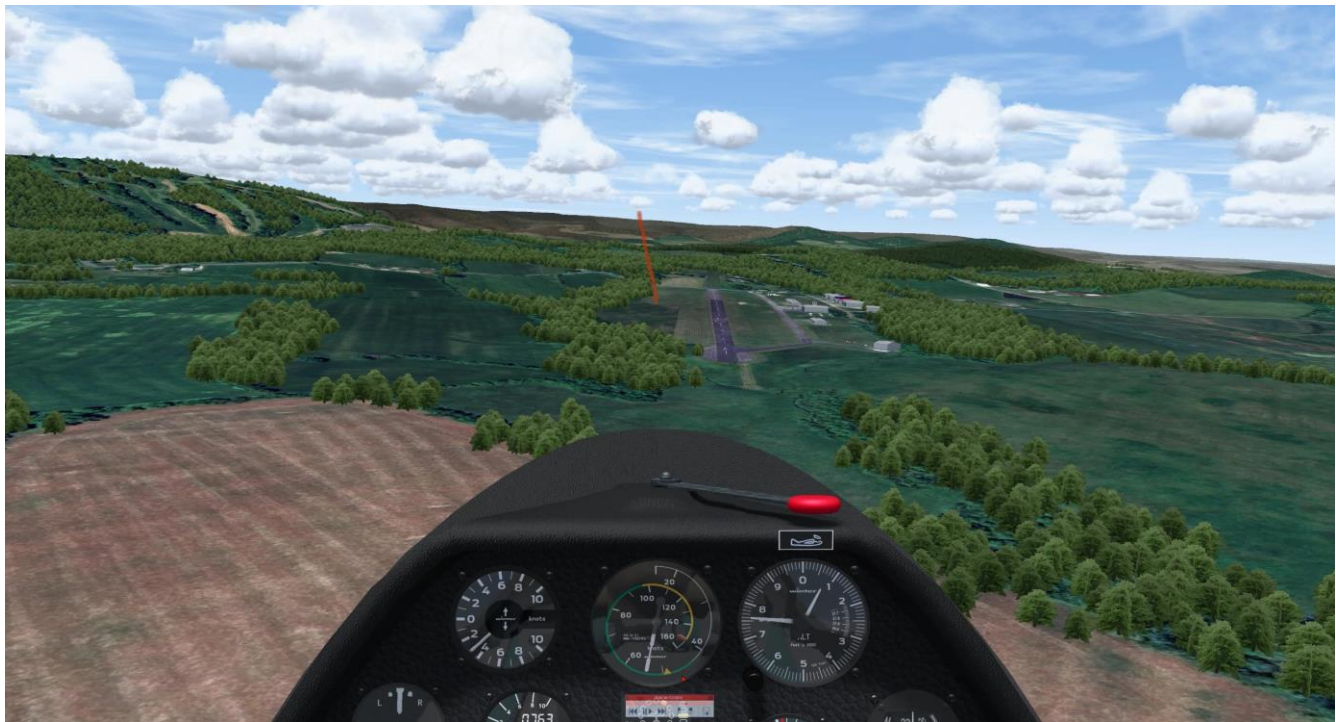
Figure 2: View of Glider turning final using PTL method – note Altimeter, ground 575.
